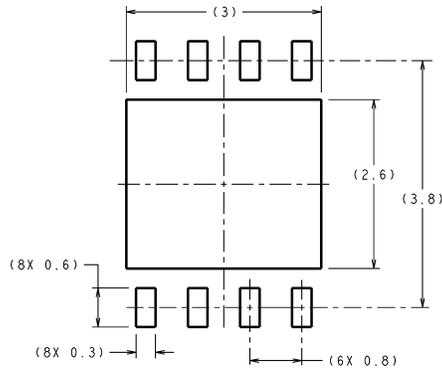
DIMENSIONS ARE IN MILLIMETERS
