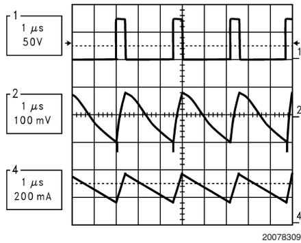
LM5007 Operation:  $V_{OUT} = 10V$ ,  $V_{IN} = 75V$ ,  $I_{OUT} = 250mA$
