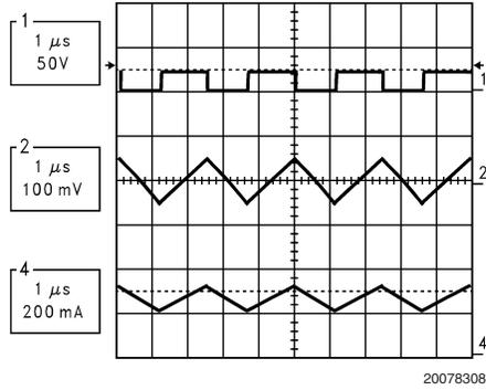
LM5007 Operation:  $V_{OUT} = 10V$ ,  $V_{IN} = 20V$ ,  $I_{OUT} = 250mA$
