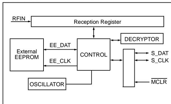
The manufacturer's code, crypt keys, and synchronization information are stored in encrypted form in external EEPROM. The HCS500 uses the S\_DAT and S\_CLK inputs to communicate with a host controller device.
