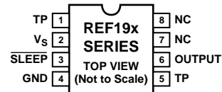
Figure 1. 8-Lead SOIC and TSSOP Pin Configuration (S Suffix and RU Suffix)
