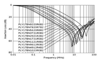
Common Mode Insertion Loss-Frequency Characteristics
