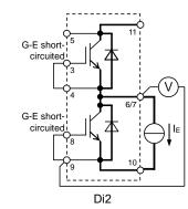
V<sub>CEsat</sub> characteristics test circuit
