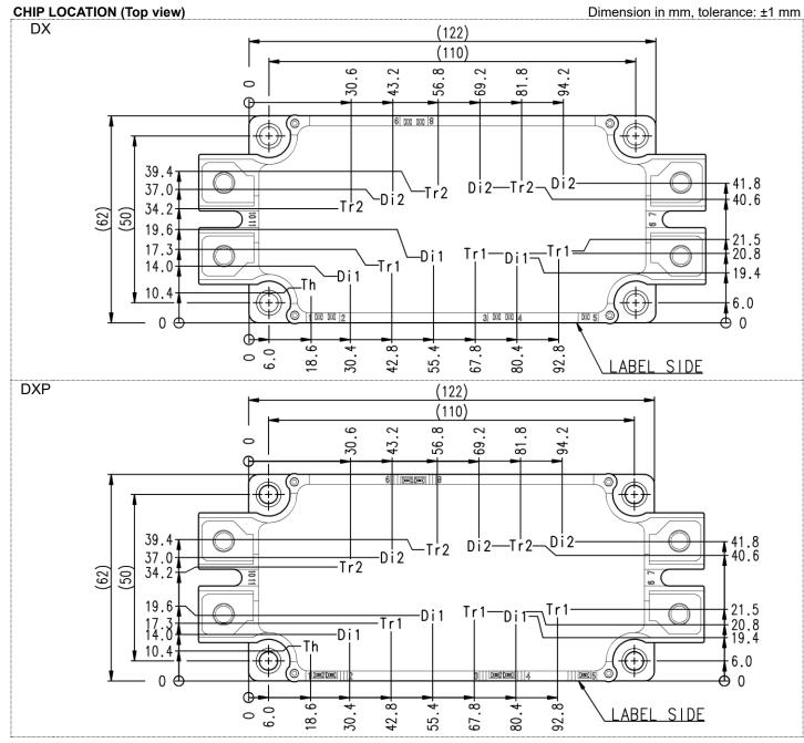
Tr1/Tr2: IGBT, Di1/Di2: FWD, Th: NTC thermistor
