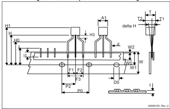
Figure 21. TO-92 ammopack mechanical data drawing
