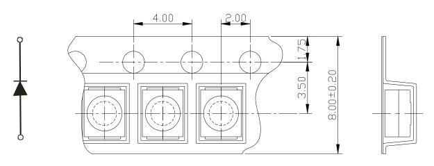
All dimensions in mm, tolerances unless mentioned is  $\pm 0.1$  mm.
