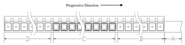
A: Top Cover Tape, 300mm; B: Leader, Empty, 200mm; C:3000 Lamps Loaded; D: Trailer, Empty, 200mm.
