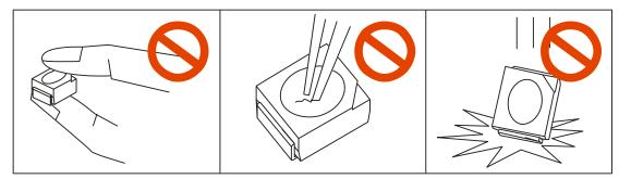
The epoxy resin of encapsulant is fragile, so please avoid scratch or friction over the epoxy resin surface. While handling the product with tweezers, do not hold by the epoxy resin, be careful.
