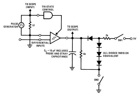
1.5V for  $t_{PHZ}$  and  $t_{PLZ}$ -1.5V for  $t_{PLZ}$  and  $t_{PZL}$ Input Pulse Characteristics:  $t_{TLH} = t_{THL} = 6$  ns (10% to 90%) PRR = 1 MHz, 50% duty cycle
