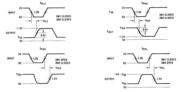
Figure 6. Propagation Delay TRI-STATE Control Unit to Output for "LS-Type" Load
