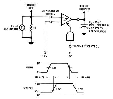
Input Pulse Characteristics:  $t_{TLH} = t_{THL} = 6$  ns (10% to 90%) PRR = 1 MHz, 50% duty cycle
