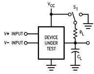
C<sub>L</sub> Includes load and test jig capacitance.
