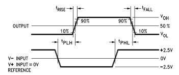
Figure 2. Propagation Delays
