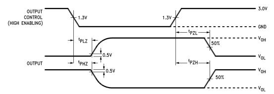
Figure 4. TRI-STATE Output Enable and Disable Waveforms
