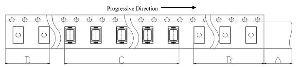
A: Top Cover Tape, 300mm; B: Leader, Empty, 200mm; C:1500 Lamps Loaded; D: Trailer, Empty, 200mm.
