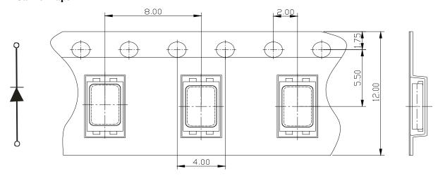
All dimensions in mm, tolerances unless mentioned is  $\pm 0.1$  mm.
