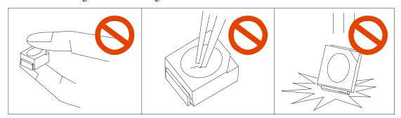
The epoxy resin of encapsulant is fragile, so please avoid scratch or friction over the epoxy resin surface. While handling the product with tweezers, do not hold by the epoxy resin, be careful.
