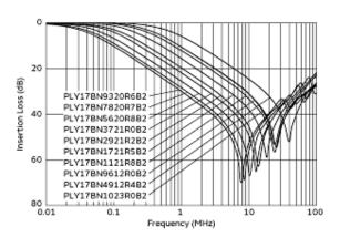
Common Mode Insertion Loss-Frequency Characteristics
