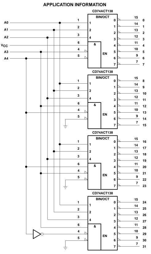
Figure 3. 32-Bit Decoding Scheme
