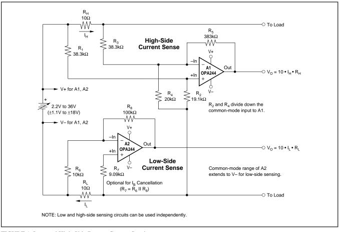
FIGURE 1. Low and High-Side Battery Current Sensing.
