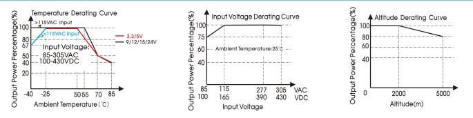
Note: 1) With an AC input between 85-115VAC and a DC input between 100-165VDC, the output power must be derated as per temperature derating curves; 2) This product is suitable for applications using natural air cooling; for applications in closed environment please consult Mornsun FAE.
