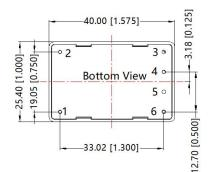
Note: Unit: mm[inch] Pin diameter tolerances: ±0.10[±0.004] General tolerances: ±0.50[±0.020]
