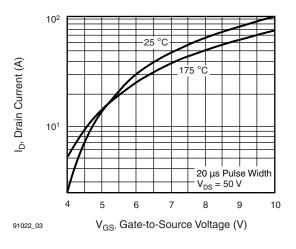
Fig. 3 - Typical Transfer Characteristics
