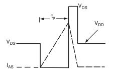
Fig. 12b - Unclamped Inductive Waveforms
