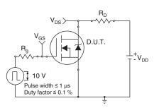
Fig. 10a - Switching Time Test Circuit
