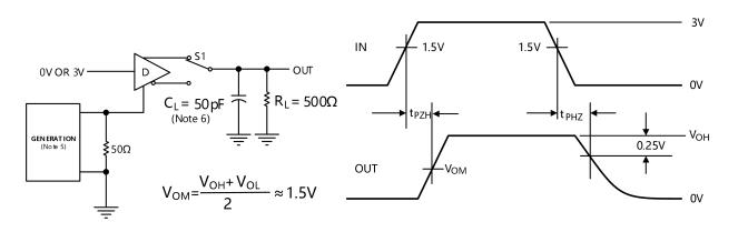
Figure 7. Driver Enable and Disable Times ( $T_{PZH}$ ,  $T_{PSH}$ ,  $T_{PHZ}$ )
