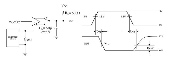
Figure 8. Driver Enable and Disable Times ( $T_{PZH}$ ,  $T_{PSH}$ ,  $T_{PHZ}$ )
