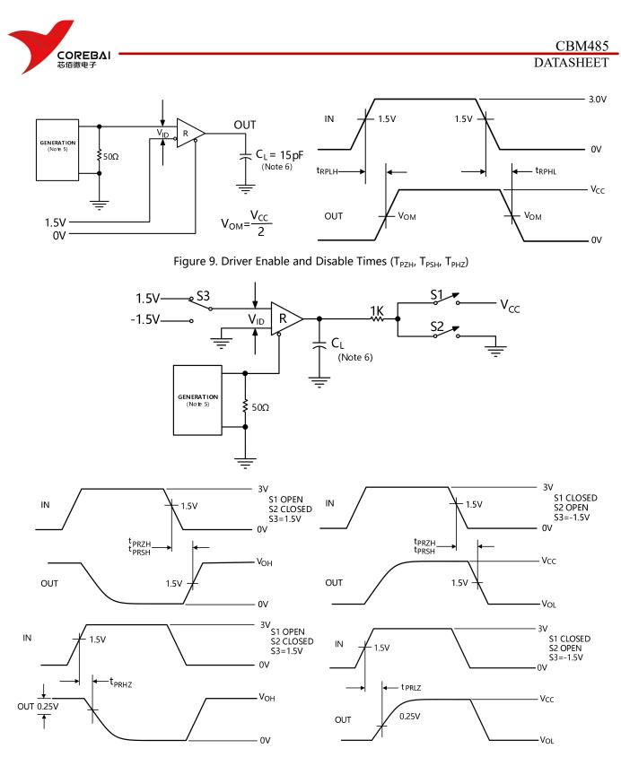
Figure 10. Driver Enable and Disable Times ( $T_{PZH}$ ,  $T_{PSH}$ ,  $T_{PHZ}$ )
