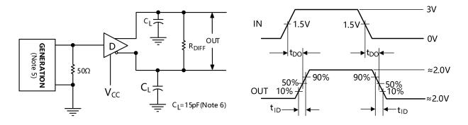
Figure 5. Driver Differential Output Delay and Transition Times
