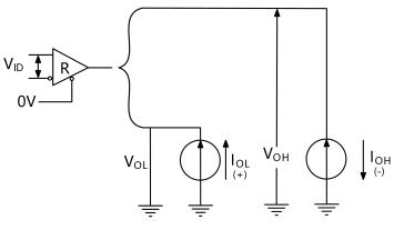
Figure 4. Receiver  $V_{OH}$  and  $V_{OL}$
