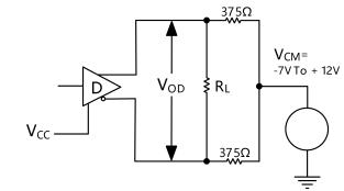
Figure 2. Driver  $V_{\text{OD}}$  and  $V_{\text{OC}}$
