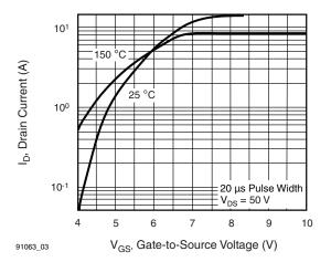
Fig. 3 - Typical Transfer Characteristics
