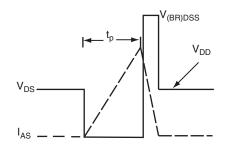
Fig. 12b - Unclamped Inductive Waveforms
