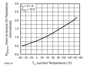
Fig. 4 - Normalized On-Resistance vs. Temperature
