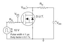
Fig. 10a - Switching Time Test Circuit
