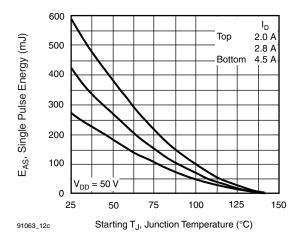
Fig. 12c - Maximum Avalanche Energy vs. Drain Current
