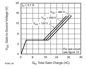
Fig. 6 - Typical Gate Charge vs. Drain-to-Source Voltage
