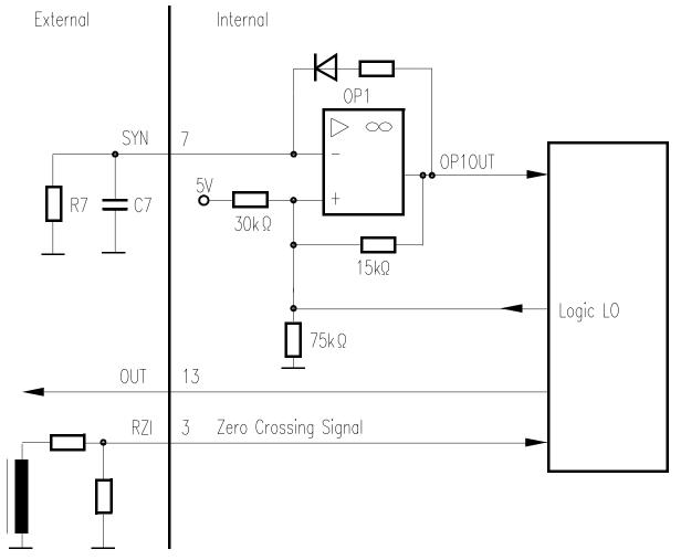
Figure 11 Synchronization and Fixed Frequency Circuit
