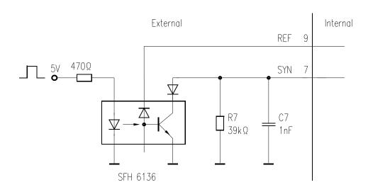
Figure 13 Ext. Synchronization Circuit
