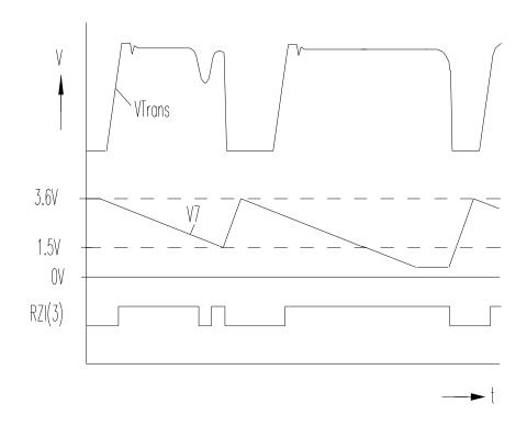
Figure 12 Pulse Diagram for Fixed Frequency Circuit
