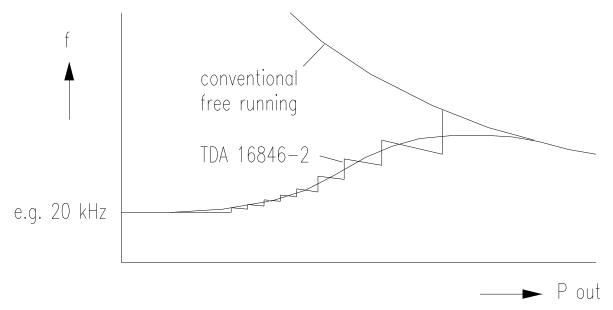
Figure 8 Load Dependent Frequency Curve
