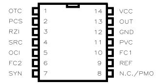
Figure 1 Pin Configuration (top view)
