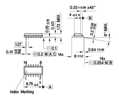
1) Does not include plastic or metal protrusion of 0.15 max. per side
