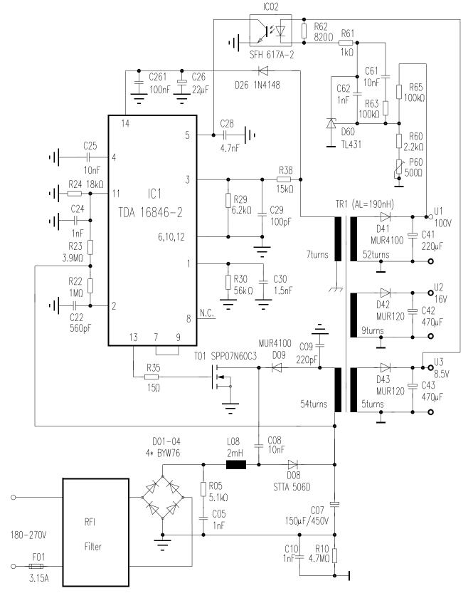
Figure 15 Circuit Diagram for Application with PFC
