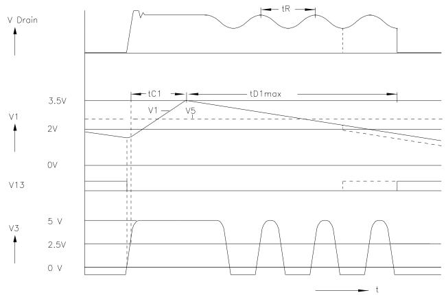
Figure 7 Pulse Diagram of Off-Time-Circuit
