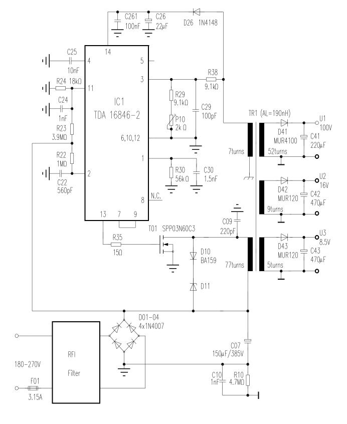
Figure 16 Circuit Diagram for Standard Application
