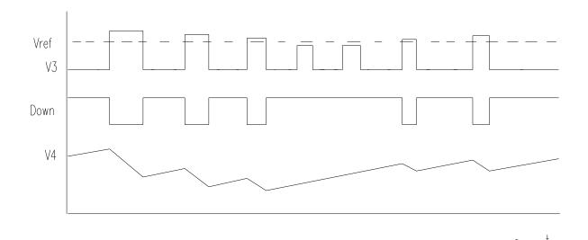
Figure 10 Regulation Pulse Diagram
