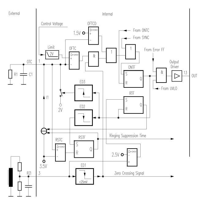
Figure 6 Off-Time-Circuit
