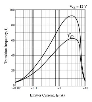
Figure 8. Transition Frequency vs. Emitter Current
