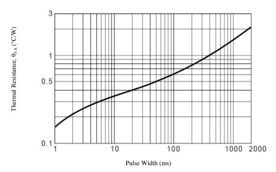
Figure 9. Transient Thermal Resistance
