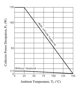
Figure 2. Power Dissipation vs. Ambient Temperature
