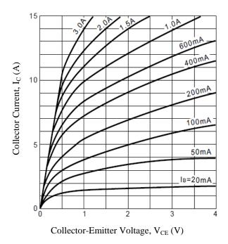
Figure 3. Collector Current vs. Collector-Emitter Voltage
