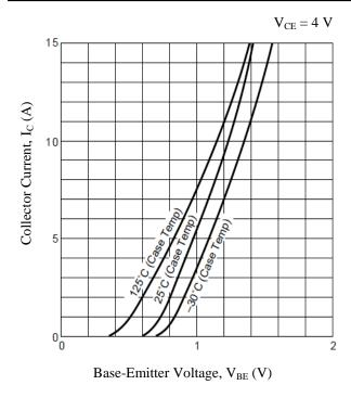
Figure 5. Collector Current vs. Base-Emitter Voltage
