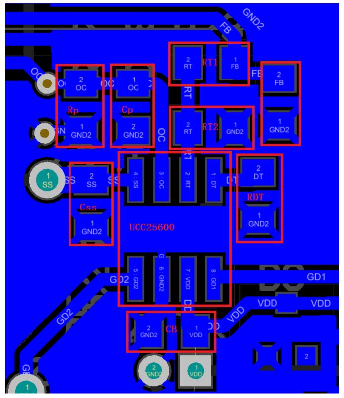
Figure 27. Board Layout Example
