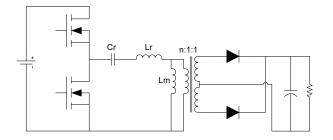
Figure 14. LLC Resonant Converter
