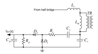
Figure 13. Current Sensing for LLC Resonant Converter
