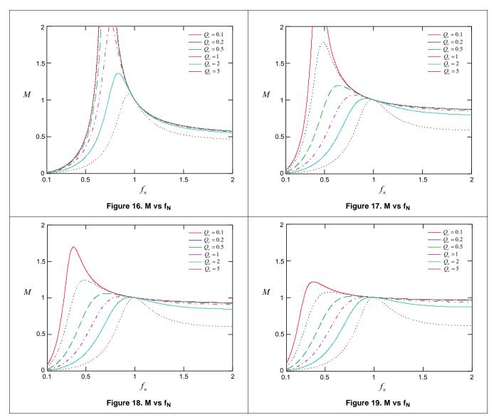
Based on its theory of operation, the LLC resonant converter is controlled through pulse frequency modulation (PFM). The output voltage is regulated by adjusting the switching frequency according to the input and output conditions. Optimal efficiency is achieved at the nominal input voltage by setting the switching frequency close to the resonant frequency. When the input voltage drops low, the switching frequency is decreased to boost the gain and maintain regulation.
