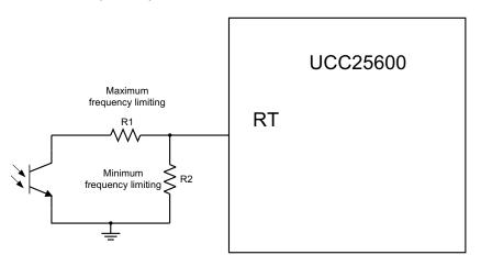
Figure 20. Maximum and Minimum Frequency Setting for UCC25600
