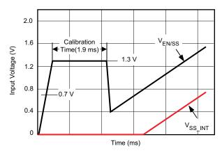
Figure 19. Startup Sequence and Timing
