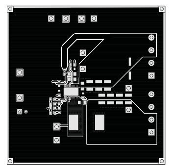
Figure 26. TPS56121EVM-601 Top Copper (Top View)
