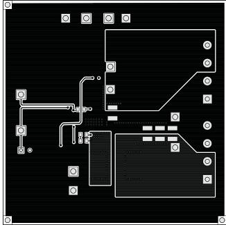
Figure 29. TPS56121EVM-601 Bottom Copper (Top View)
