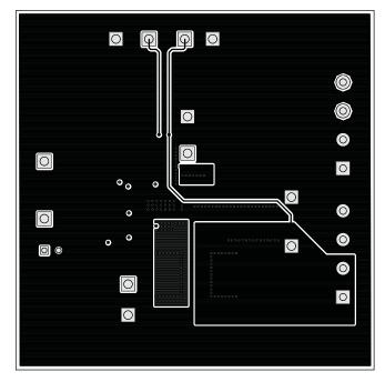
Figure 28. TPS56121EVM-601 Internal 2 (Top View)
