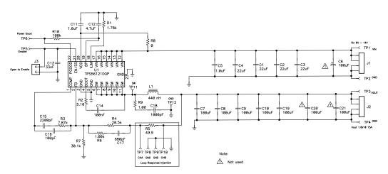
Figure 20. Design Example Schematic
