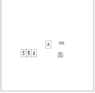
Figure 24. TPS56121EVM-601 Top Assembly Drawing (Top view)
