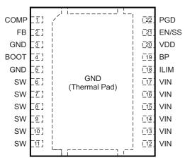
Note: The thermal pad is also an electrical ground connection.
