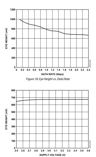
Figure 19. Eye Height vs. Supply Voltage
