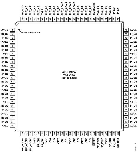
Figure 3. Pin Configuration
