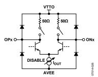
Figure 26. High Speed Output Simplified Schematic
