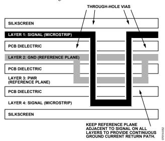
Figure 32. Example Routing of Reference Plane
