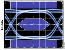
**0.125UI/DIV AT 2.25Gbps** Figure 10. Tx Eye Diagram at TP2, PE = 2 dB
