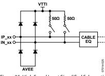
Figure 25. High Speed Input Simplified Schematic
