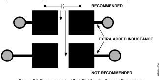
Figure 34. Recommended Pad Outline for Bypass Capacitors
