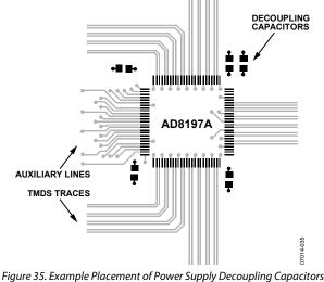
ire 35. Example Placement of Power Supply Decoupling Capacito Around the AD8197A
