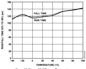
Figure 22. Rise and Fall Time vs. Temperature
