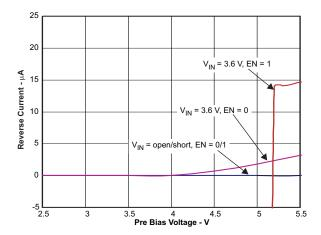
Figure 6. Reverse Current Test Results (Typical)
