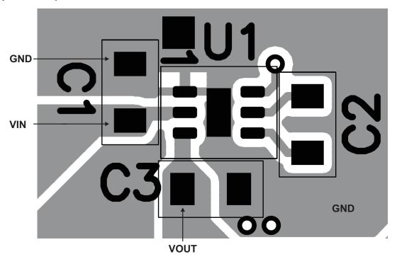
Figure 27. Recommended PCB Layout
