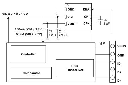
Figure 10. Application Circuit for OTG System
