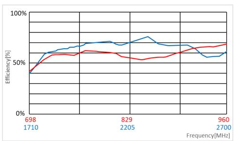
Data measured in free space and on plastic device enclosure
