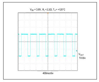
Figure 4. Cycled Output During Continuous Thermal Overload Condition
