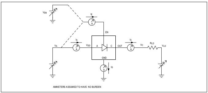
Figure 2. Ideal Diode Test Setup and Naming Convention
