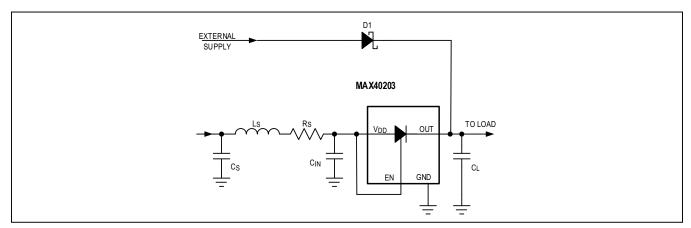
Figure 3. Typical OR Application Showing Source Impedance
