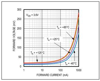
Figure 1. Forward Voltage vs. Forward Current
