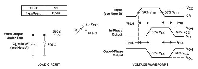
NOTES: A. C<sub>I</sub> includes probe and jig capacitance.
