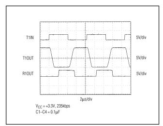
Figure 10. Loopback Test Result at 235kbps
