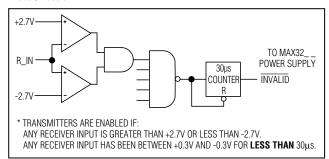
Figure 3b. MAX32\_ with Transmitters Enabled Using AutoShutdown
