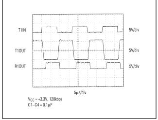
Figure 9. Loopback Test Result at 120kbps
