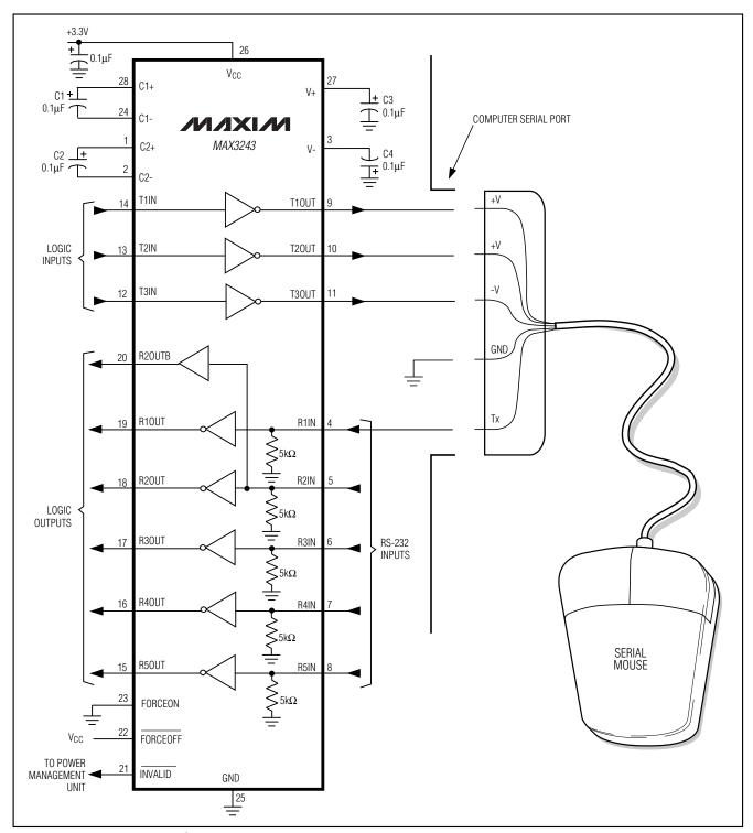
Figure 7b. Mouse Driver Test Circuit
