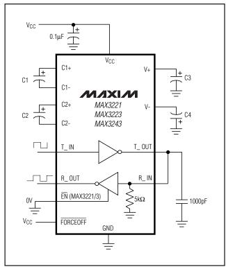
Figure 8. Loopback Test Circuit
