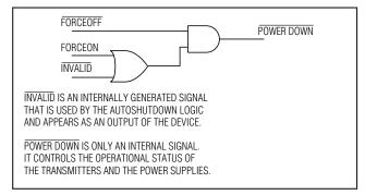
Figure 3c. AutoShutdown Logic
