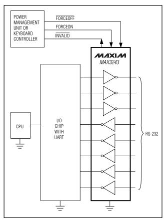
Figure 1. Interface Under Control of PMU
