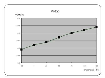
Figure 3. Start Threshold Voltage
