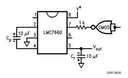
FIGURE 4. Synchronizing to an External Clock
