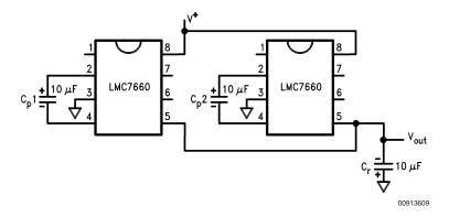
FIGURE 5. Lowering Output Resistance by Paralleling Devices
