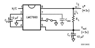
FIGURE 1. LMC7660 Test Circuit
