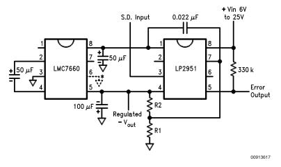
$$V_{out} = V_{ref} \left( 1 + \frac{R1}{R2} \right)$$
