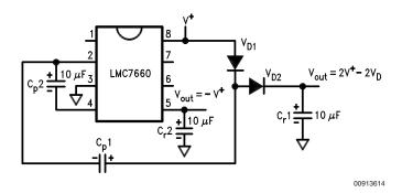
FIGURE 10. Combined Negative Converter and Positive Multiplier
