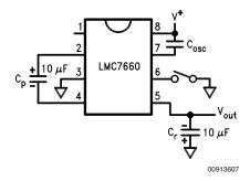
FIGURE 3. Reduce Supply Current by Lowering Oscillator Frequency
