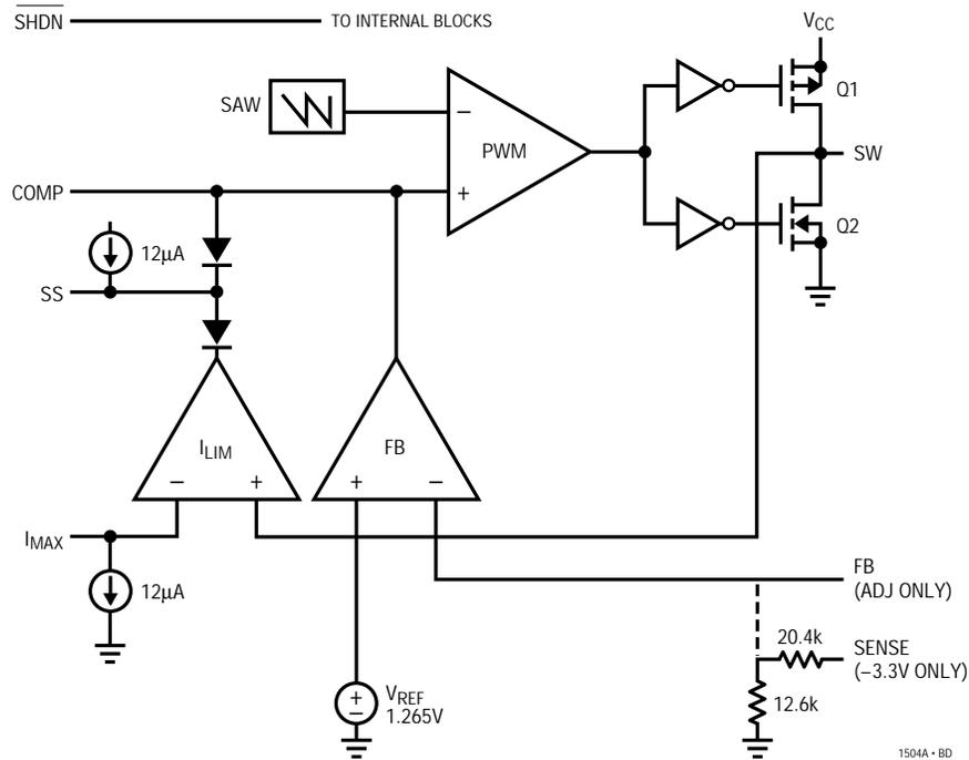
Figure 3. Block Diagram
