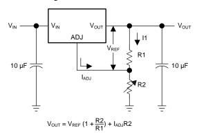
Figure 3. Basic Adjustable Regulator
