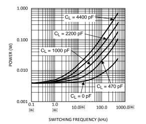
Figure 18. Gate Driver Power Dissipation (LO + HO)  $V_{CC}$  = 12V, Neglecting Diode Losses
