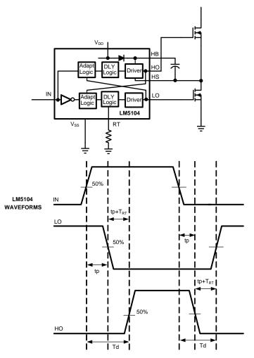
Figure 16. Application Timing Waveforms
