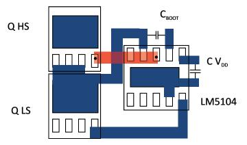
Figure 21. LM5104 Component Placement
