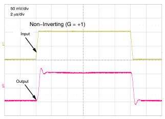
Figure 22. Step Response – Small Signal
