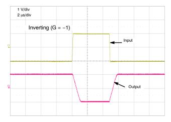
Figure 25. Step Response – Large Signal
