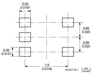
NOTES: 1. DIMENSIONING AND TOLERANCING PER ANSI Y14.5M, 1982. 2. CONTROLLING DIMENSION: INCH. 3. 419A-01 OBSOLETE. NEW STANDARD 419A-02. 4. DIMENSIONS A AND B DO NOT INCLUDE MOLD FLASH, PROTRUSIONS, OR GATE BURRS.
