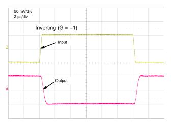
Figure 23. Step Response – Small Signal
