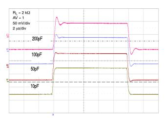
Figure 20. Settling Time vs. Capacitive Load
