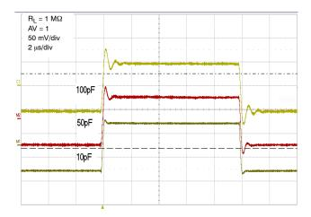
Figure 21. Settling Time vs. Capacitive Load
