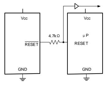
Figure 2. Buffered RESET to other system components
