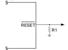
Figure 1. RESET Valid to Ground Circuit
