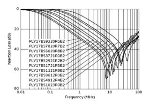
Common Mode Insertion Loss-Frequency Characteristics
