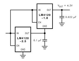
Figure 24. Stacking Voltage References Circuit
