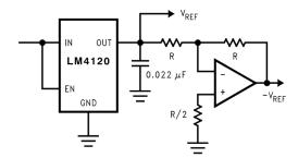
Figure 22. Voltage Reference With Complimentary Output Circuit
