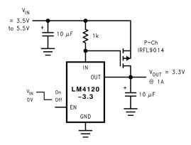
Figure 23. Precision High-Current Low-Dropout Regulator Circuit
