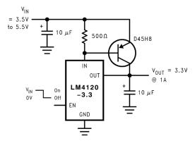
Figure 20. Precision High-Current Low-Dropout Regulator Circuit
