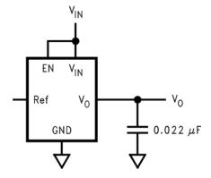
Figure 29. Standard Application Circuit
