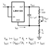
Figure 26. Programmable Current Source Circuit
