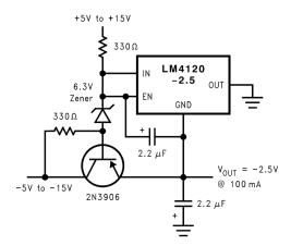
Figure 21. Precision High-Current Negative Voltage Regulator Circuit
