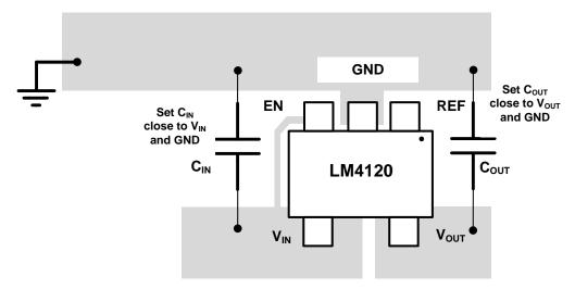
Figure 32. Typical Layout Example With LM4120
