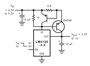
Figure 27. Precision Regulator With Current Limiting Circuit
