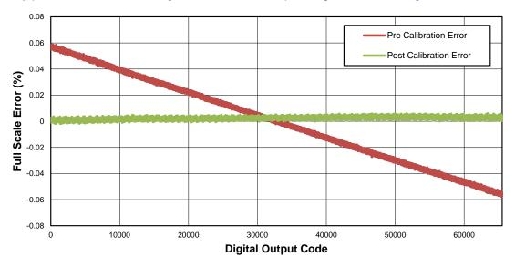
Figure 98. System Accuracy Performance in ±2.5 x V<sub>REF</sub> Input Range
