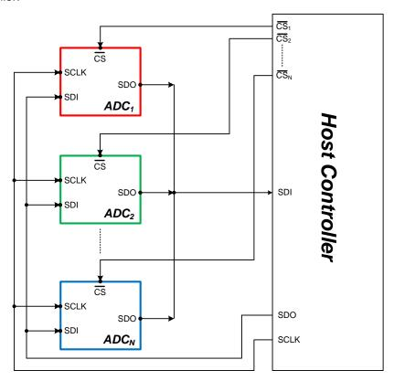
Figure 75. Star Topology Connection Schematic
