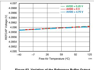
Figure 63. Variation of the Reference Buffer Output (REFCAP) Across Supply and Temperature
