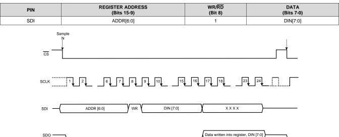
Figure 88. Program Register Write Cycle Timing Diagram
