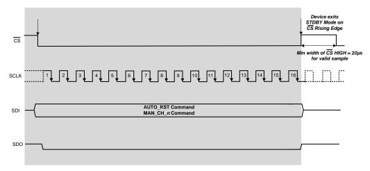
Figure 78. Exit STDBY Mode Timing Diagram
