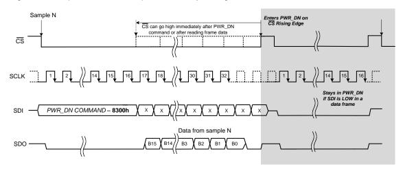
Figure 79. Enter and Remain in PWR DN Mode Timing Diagram
