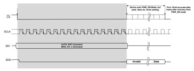
Figure 80. Exit PWR\_DN Mode Timing Diagram
