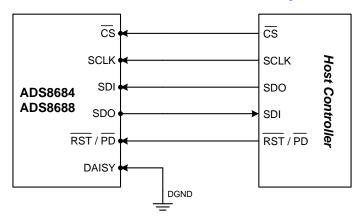
Figure 70. Pin Configuration for the Digital Interface
