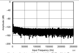
Number of points = 64k,  $f_{IN} = 1$  kHz, SNR = 91.4 dB, SINAD = 91.2 dB, THD = 105 dB, SFDR = 107 dB
