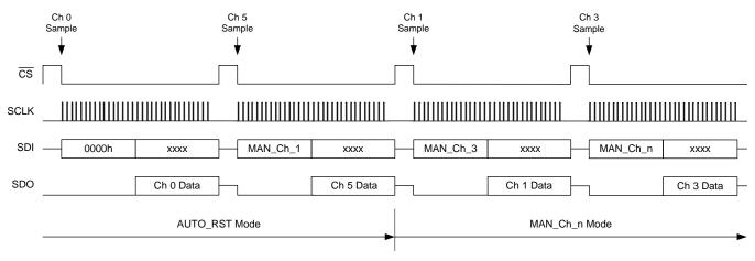
Figure 85. Transitioning from AUTO\_RST to MAN\_Ch\_n Mode (Channels 0 and 5 are Selected for Auto Sequence)
