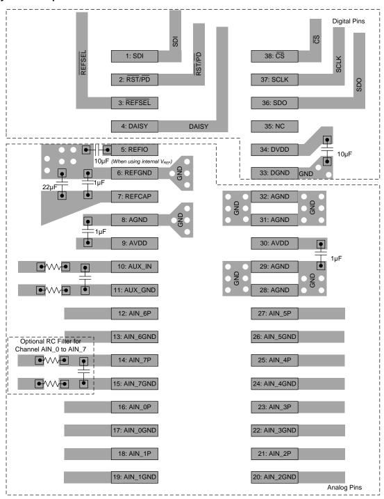
Figure 101. Board Layout for the ADS8684 and ADS8688
