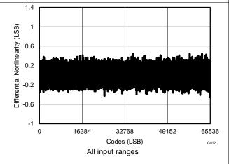
Figure 10. DC Histogram for Mid-Scale Inputs (1.25  $\times$  V<sub>REF</sub>)
