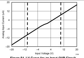
Figure 54. I-V Curve for an Input OVP Circuit
