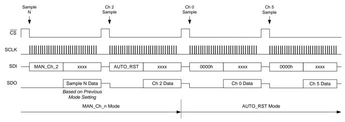
Figure 86. Transitioning from MAN\_Ch\_n to AUTO\_RST Mode (Channels 0 and 5 are Selected for Auto Sequence)
