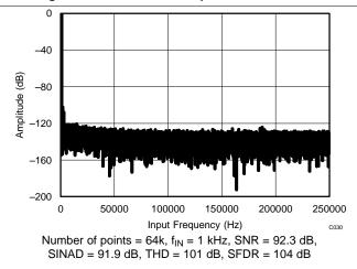
Figure 30. Typical FFT Plot (±2.5 × V<sub>REF</sub>)
