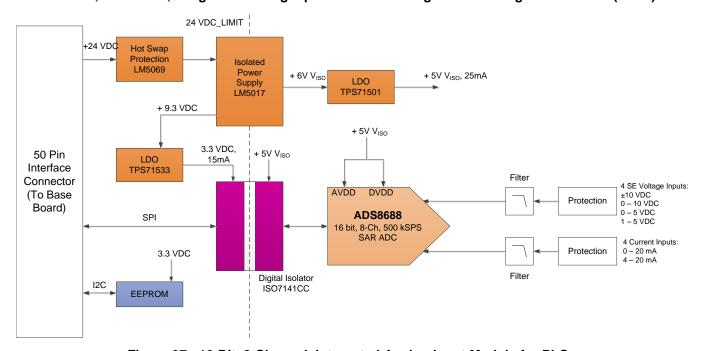
Figure 97. 16-Bit, 8-Channel, Integrated Analog Input Module for PLCs
