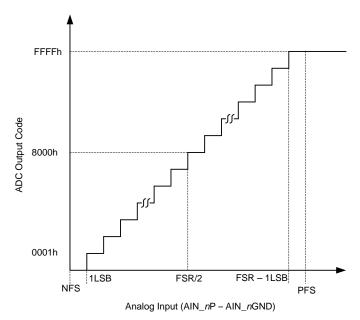
Figure 69. 16-Bit ADC Transfer Function (Straight Binary Format)
