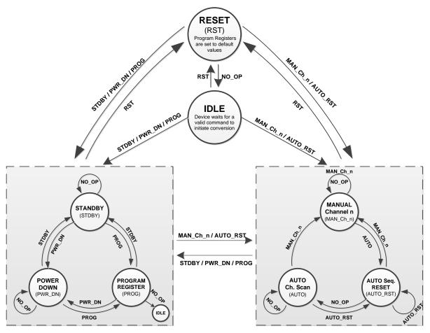
Figure 76. State Transition Diagram
