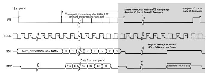
Figure 81. Enter AUTO\_RST Mode Timing Diagram
