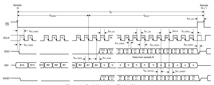
Figure 1. Serial Interface Timing Diagram
