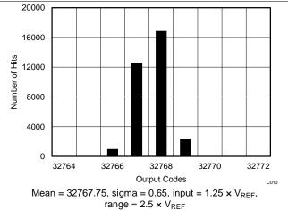
Figure 8. DC Histogram for Mid-Scale Inputs ( $\pm 0.625 \times V_{REF}$ )
