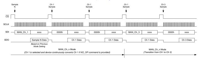
Figure 84. Device Operation in MAN\_Ch\_n Mode
