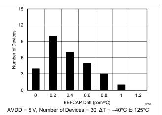
Figure 64. Reference Buffer Temperature Drift Histogram
