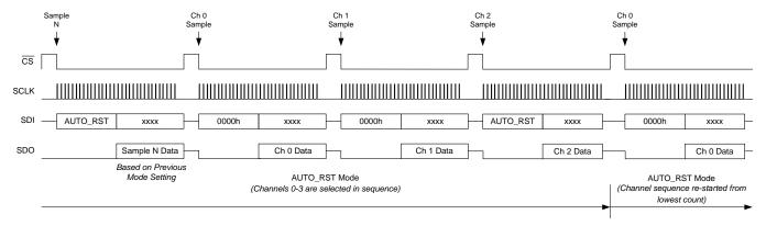
Figure 82. Device Operation Example in AUTO RST Mode
