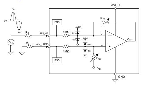
Figure 52. Input Overvoltage Protection Circuit Schematic
