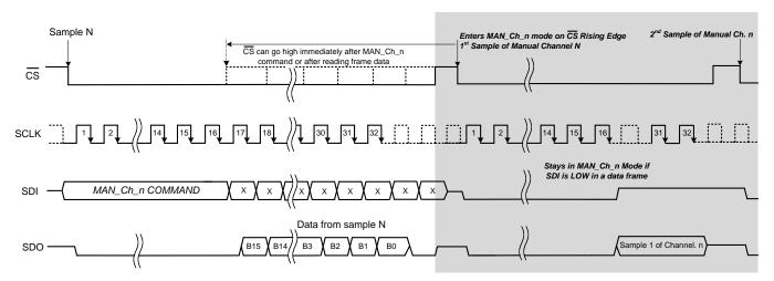
Figure 83. Enter MAN Ch n Scan Mode Timing Diagram
