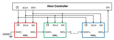
Figure 73. Daisy-Chain Connection Schematic
