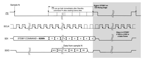
Figure 77. Enter and Remain in STDBY Mode Timing Diagram
