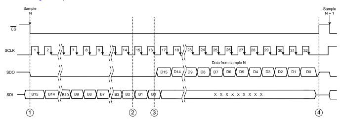
Figure 72. Device Operation Using the Serial Interface Timing Diagram
