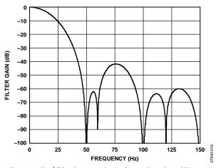
Figure 24. Sinc<sup>3</sup> Filter Response (50 Hz Output Data Rate, REJ60 = 1)
