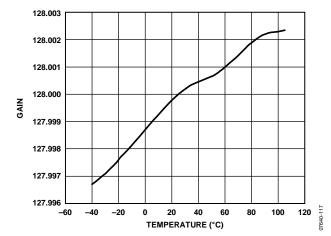
Figure 17. Gain Error (Gain = 128, Chop Disabled)
