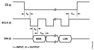
Figure 4. Write Cycle Timing Diagram
