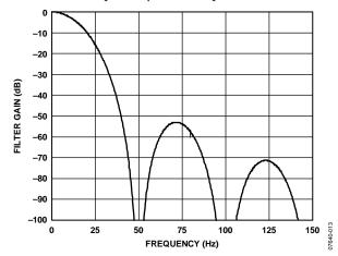
Figure 19. Sinc<sup>4</sup> Filter Response (50 Hz Output Data Rate)
