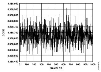
Figure 8. Noise ( $V_{REF} = 5 V$ , Output Data Rate = 4800 Hz, Gain = 128, Chop Disabled, Sinc<sup>4</sup> Filter)
