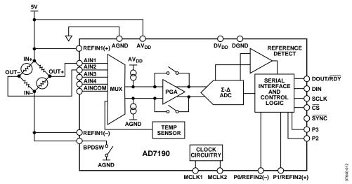
Figure 18. Basic Connection Diagram
