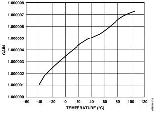
Figure 16. Gain Error (Gain = 1, Chop Disabled)
