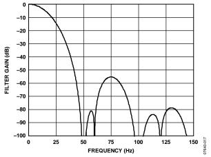
Figure 23. Sinc⁴ Filter Response (50 Hz Output Data Rate, REJ60 = 1)
