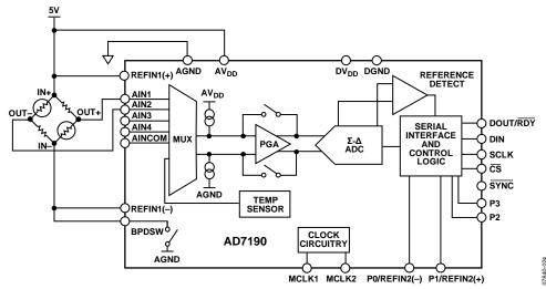
Figure 32. Typical Application (Weigh Scale)
