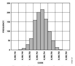
Figure 7. Noise Distribution Histogram ( $V_{REF} = 5 V$ , Output Data Rate = 4.7 Hz, Gain = 128, Chop Disabled, Sinc<sup>4</sup> Filter)
