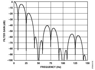
Figure 22. Sinc<sup>3</sup> Filter Response (Output Data Rate = 16.6 Hz, Chop Enabled)
