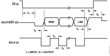
Figure 3. Read Cycle Timing Diagram
