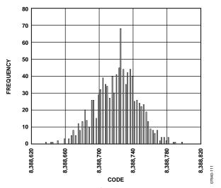
Figure 11. Noise Distribution Histogram ( $V_{REF} = 5 V$ , Output Data Rate = 4800 Hz, Gain = 1, Chop Disabled, Sinc<sup>4</sup> Filter)
