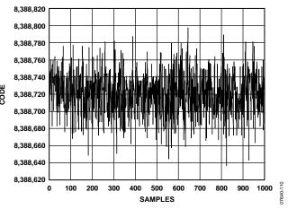
Figure 10. Noise (V<sub>REF</sub> = 5 V, Output Data Rate = 4800 Hz, Gain = 1, Chop Disabled, Sinc<sup>4</sup> Filter)
