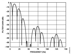
Figure 21. Sinc⁴ Filter Response (Output Data Rate = 12.5 Hz, Chop Enabled)
