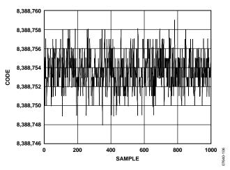
Figure 6. Noise ( $V_{REF} = 5 V$ , Output Data Rate = 4.7 Hz, Gain = 128, Chop Disabled, Sinc<sup>4</sup> Filter)
