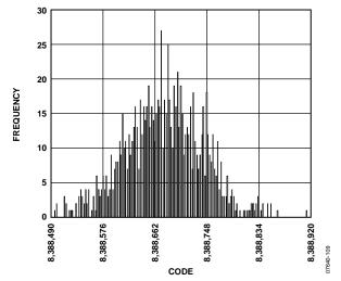
Figure 9. Noise Distribution Histogram ( $V_{REF} = 5 V$ , Output Data Rate = 4800 Hz, Gain = 128, Chop Disabled, Sinc<sup>4</sup> Filter)
