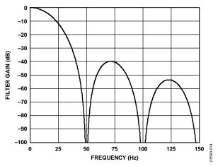
Figure 20. Sinc<sup>3</sup> Filter Response (50 Hz Output Data Rate)
