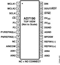
Figure 5. Pin Configuration
