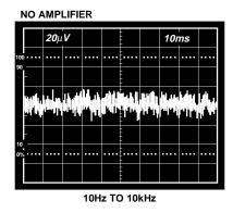
Figure 6. Reduced Noise Performance with C1 =  $100 \, \mu F$ , C2 =  $100 \, nF$
