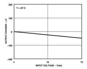
Figure 14. Output Voltage Change vs. Input Voltage
