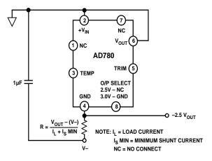
Figure 18. Negative (-2.5 V) Shunt Mode Reference
