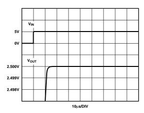
Figure 11. Turn-On Settling Time Performance
