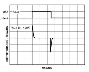
Figure 12b. Settling Under Transient Resistive Load
