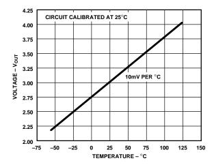
Figure 8. Temperature Pin Transfer Characteristic
