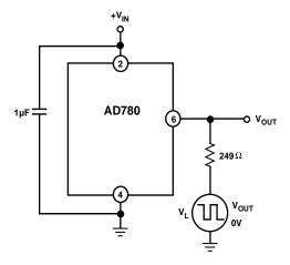
Figure 12a. Transient Resistive Load Test Circuit
