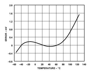
Figure 7. Typical AD780BN Temperature Drift
