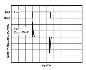
Figure 13b. Settling Under Dynamic Capacitive Load
