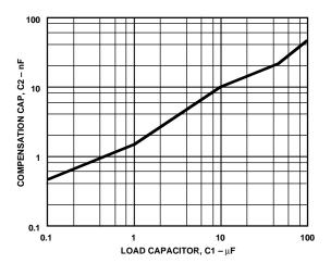
Figure 3. Compensation and Load Capacitor Combinations
