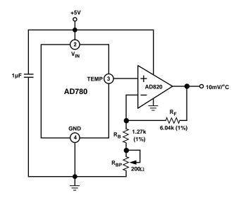
Figure 9. Differential Temperature Transducer
