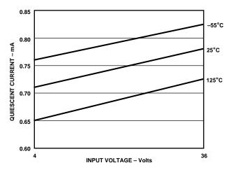
Figure 10. Typical Supply Current over Temperature
