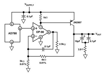
Figure 17. +4.5 V Reference from a Single +5 V Supply
