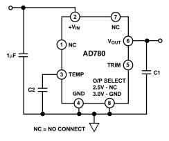
Figure 5. Noise Reduction Circuit
