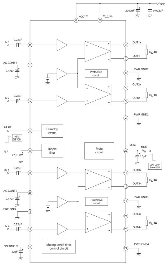
Note : The components and constant values in the test circuit are used for confirmation of characteristics and do not guarantee that the application equipment will be free from malfunction or trouble
