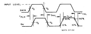
Fig. 3 - Data to Qn output propagation delays.
