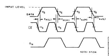
Fig. 5 - Latch enable prerequisite times.
