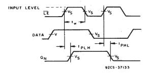
Fig. 4 - Latch enable propagation delays.
