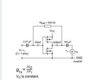
Fig. 9. Test set-up for measuring forward transconductance
