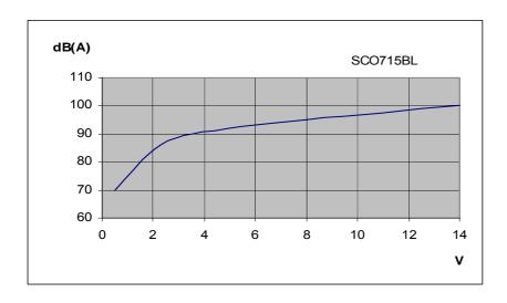
All measurements are made at 1 meter in free air at 21°C.
