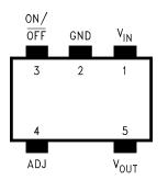
Figure 1. 5-Lead Small Outline Package Top View See Package Number DBV0005A
