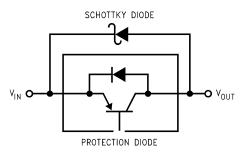
Figure 22. Adding External Schottky Diode Protection
