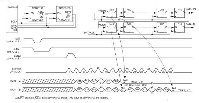
Figure 28. Timing of TAG Feature With Single Conversion (Using External DATACLK)
