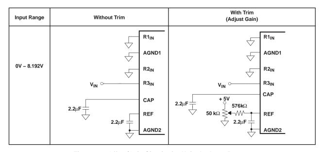
Figure 29. Offset/Gain Circuits for Unipolar Input Ranges
