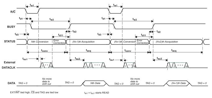
Figure 3. Basic Conversion Timing: External DATACLK
