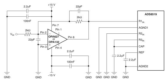
Figure 31. Typical Driving Circuitry (±10V, No Trim)
