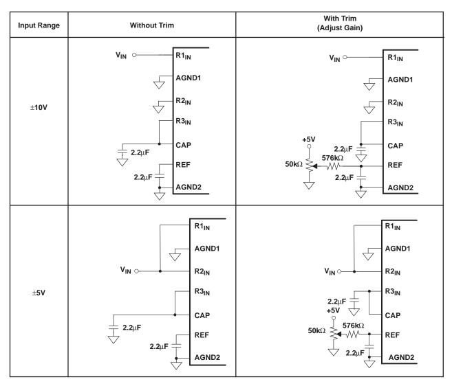
Figure 30. Offset/Gain Circuits for Bipolar Input Ranges
