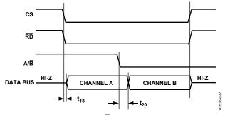
Figure 28.  $A/\overline{B}$  Channel Reading
