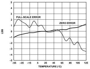
Figure 14. Full-Scale Error and Zero Error vs. Temperature
