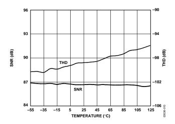
Figure 11. SNR, THD vs. Temperature
