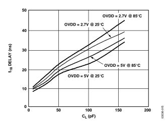
Figure 16. Typical Delay vs. Load Capacitance C<sub>L</sub>
