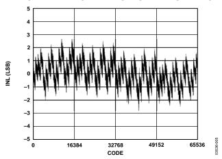
Figure 6. Integral Nonlinearity vs. Code
