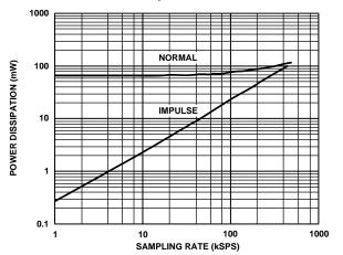
Figure 21. Power Dissipation vs. Sample Rate
