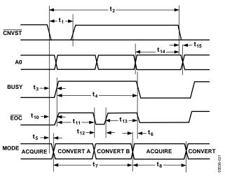
Figure 22. Basic Conversion Timing
