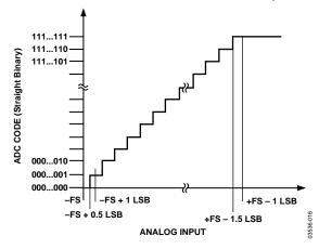
Figure 17. ADC Ideal Transfer Function
