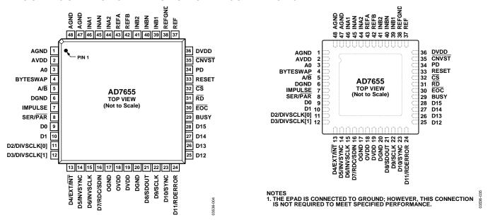
Figure 4. 48-Lead LQFP Pin Configuration
