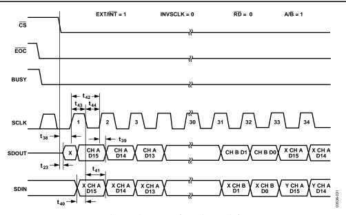
Figure 32. Slave Serial Data Timing for Reading (Read After Convert)
