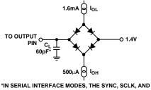
SDOUT TIMINGS ARE DEFINED WITH A MAXIMUM LOAD  $C_L$  OF 10pF; OTHERWISE, THE LOAD IS 60pF MAXIMUM.
