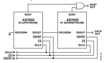
Figure 31. Two AD7655 Devices in a Daisy-Chain Configuration
