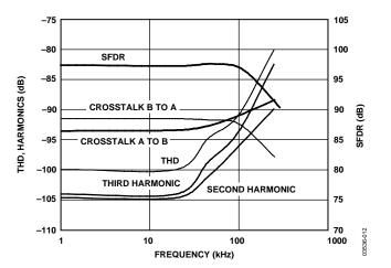
Figure 13. THD, Harmonics, Crosstalk, and SFDR vs. Frequency
