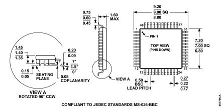
Figure 35. 48-Lead Low Profile Quad Flat Package [LQFP] (ST-48)
