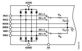
Figure 19. Simplified Analog Input
