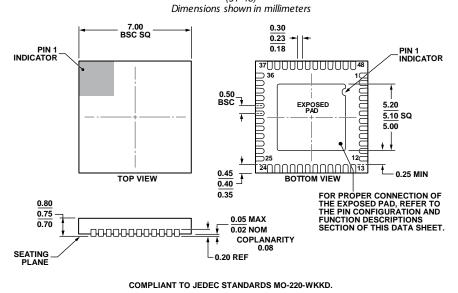
Figure 36. 48-Lead Lead Frame Chip Scale Package [LFCSP] 7 mm × 7 mm Body and 0.75 mm Package Height (CP-48-4) Dimensions shown in millimeters
