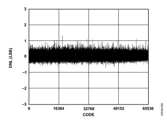
Figure 9. Differential Nonlinearity vs. Code
