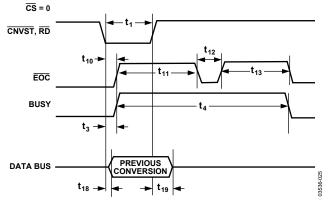
Figure 26. Slave Parallel Data Timing for Reading (Read During Convert)
