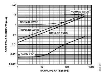
Figure 15. Operating Currents vs. Sample Rate
