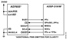
Figure 34. Interfacing the AD7655 to SPI Interface
