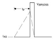
Fig 12b. Unclamped Inductive Waveforms
