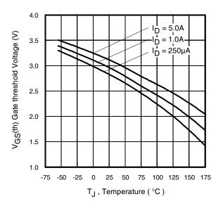
Fig 14. Threshold Voltage Vs. Temperature
