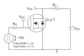
Fig 18a. Switching Time Test Circuit
