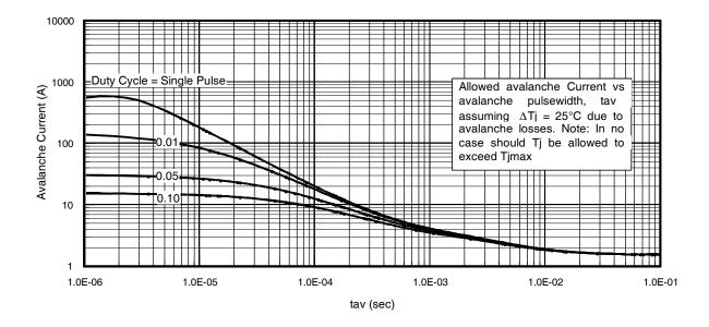
Fig 15. Typical Avalanche Current Vs.Pulsewidth
