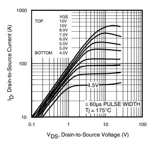
Fig 2. Typical Output Characteristics
