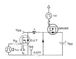
Fig 12a. Unclamped Inductive Test Circuit
