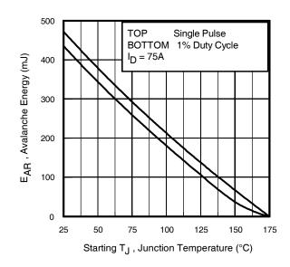
Fig 16. Maximum Avalanche Energy Vs. Temperature
