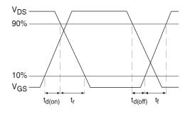
Fig 18b. Switching Time Waveforms
