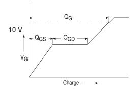
Fig 13a. Basic Gate Charge Waveform
