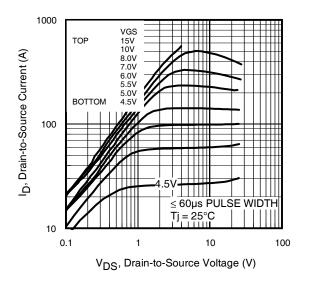
Fig 1. Typical Output Characteristics
