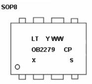
C: SOP8 Package P: Pb-free Package Y: Year Code(0-9) WW: Week Code(01-52) X: Version s: Internal Code
