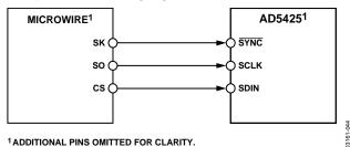
Figure 43. MICROWIRE to AD5425 Interface
