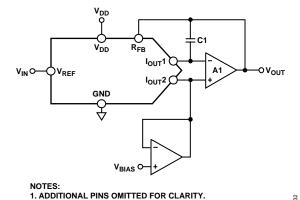
Figure 32. Single-Supply Current Mode Operation
