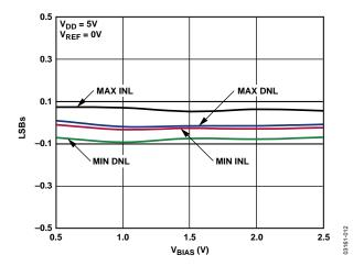
Figure 12. Linearity vs.  $V_{\text{BIAS}}$  Voltage Applied to  $I_{\text{OUT}}2$
