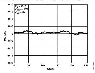
Figure 4. Integral Nonlinearity (INL) vs. Code (8-Bit DAC)
