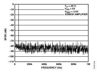
Figure 24. Wideband SFDR, Clock = 2 MHz,  $f_{OUT}$  = 50 kHz
