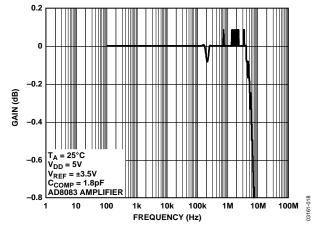
Figure 18. Reference Multiplying Bandwidth—All 1s Loaded
