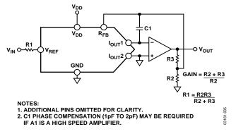
Figure 34. Increasing the Gain of Current Output DAC
