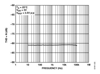
Figure 22. THD and Noise vs. Frequency
