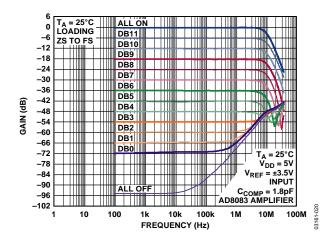
Figure 20. Reference Multiplying Bandwidth vs. Frequency and Code
