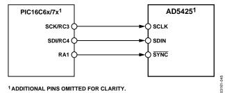
Figure 44. PIC16C6x/PIC16C7x to AD5425 Interface
