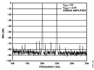
Figure 28. Narrow-Band IMD ( $\pm 50\%$ ) Clock = 2 MHz,  $f_{\rm OUT}1=20$  kHz,  $f_{\rm OUT}2=25$  kHz
