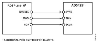
Figure 37. ADSP-2191M SPI to AD5425 Interface
