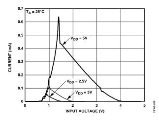
Figure 16. Supply Current vs. Input Voltage
