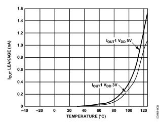
Figure 8. Ιουτ1 Leakage Current vs. Temperature
