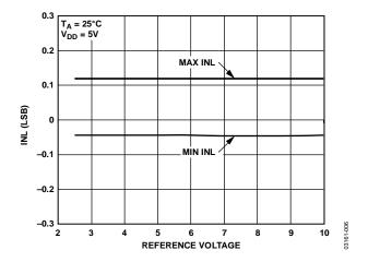
Figure 6. INL vs. Reference Voltage
