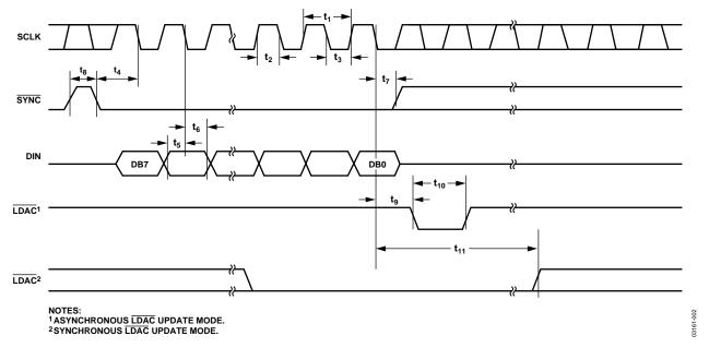
Figure 2. Timing Diagram
