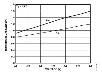
Figure 17. Threshold Voltages vs. Supply Voltage
