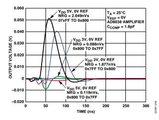
Figure 19. Midscale Transition,  $V_{REF} = 3.5 V$
