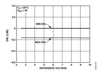
Figure 7. DNL vs. Reference Voltage
