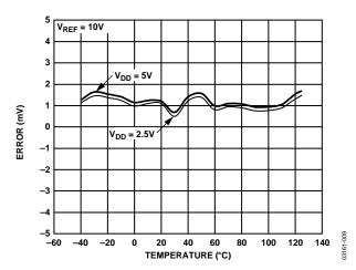
Figure 9. Gain Error vs. Temperature
