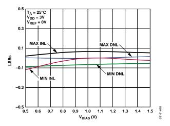
Figure 10. Linearity vs. V<sub>BIAS</sub> Voltage Applied to I<sub>OUT</sub>2
