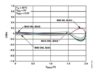
Figure 15. Linearity vs. V<sub>BIAS</sub> Voltage Applied to I<sub>OUT</sub>2
