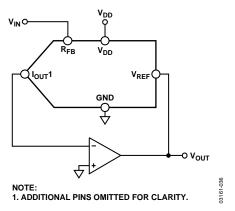
Figure 35. Current Steering DAC Used as a Divider or Programmable Gain Element
