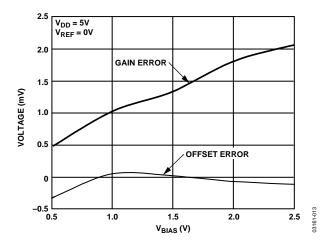
Figure 13. Gain and Offset Errors vs. Voltage Applied to Ιουτ2
