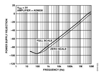
Figure 23. Power Supply Rejection vs. Frequency
