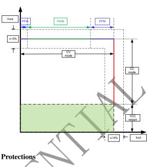
BP3519 offers rich protections to improve the system reliability, including output overvoltage protection, load short protection, Vcc under voltage lock out protection, over temperature protection.
