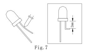
2) Forming lead should be carried our prior to soldering and never during or after soldering.
